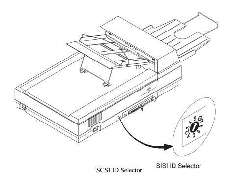
Figure 2-3 Adjusting the SCSI ID setting.
